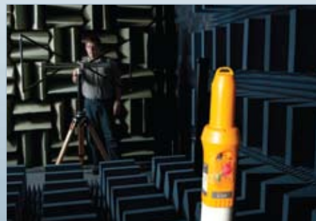
RF Anechoic testing chamber
