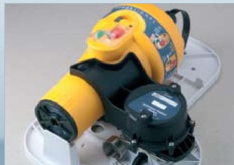
EPIRB Mounted with hydrostatic release
